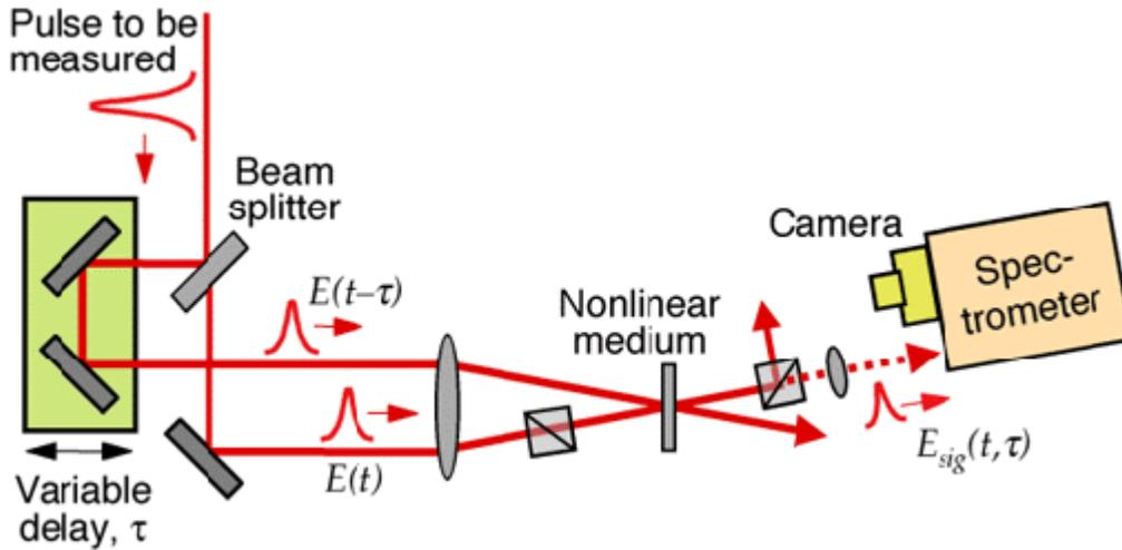
Fig. 4. FROG apparatus using the polarization-gate beam geometry.
