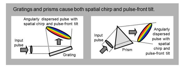
Fig. 2. Dispersive elements can yield both spatial chirp and pulse-front tilt. Pulse compressors, which are composed of as many as four dispersive elements, can yield both of these distortions unless aligned perfectly.
