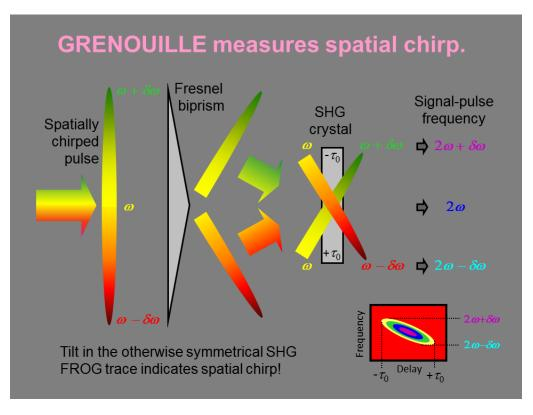
Fig. 3. A pulse with spatial chirp entering a GRENOUILLE. The Fresnel biprism separates the bluer and redder halves of the beam, which cross in the SHG crystal. Notice that the mean wavelength will vary across the trace, indicating the spatial chirp.
