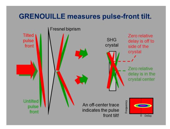
Fig. 4. Pulses with (red) and without (green) pulse-front tilt entering a GRENOUILLE. Notice that pulse-front tilt displaces the trace center by an amount directly proportional to the pulse-front tilt.
