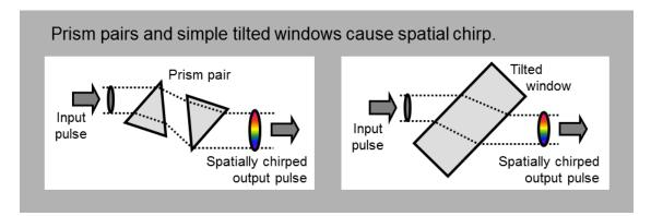
Fig. 1. Passage through a pair of prisms or a tilted window causes spatial chirp (due to Snell's law).
