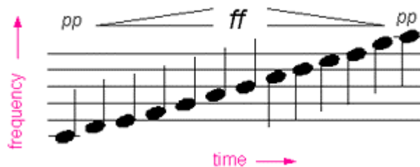
Fig. 1. The musical score is a plot of an acoustic waveform's frequency vs. time, with information on top regarding the intensity. Here the wave increases in frequency with time. It also begins at low intensity (pianissimo), increases to a high intensity (fortissimo), and then decreases again. Musicians call this waveform a "scale," but ultrafast laser scientists refer to it as a "linearly chirped pulse."
